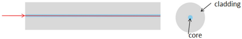
Fig.5. 8: Structure of monomode or single-mode optical fiber
