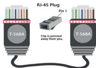
Picture 3.8: Wiring Schemes T568A
