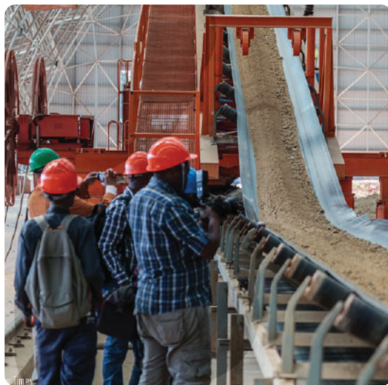
Fig 16.4 Cement on a conveyor belt at the CIMERWA Cement Factory
