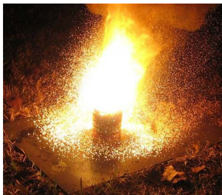
Figure 5.1: The displacement reaction between iron (III) oxide and powdered aluminium produces so much heat that iron metal is obtained in molten form.
