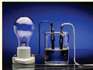
Pure water, \text{H}_2\text{O}(l) does not conduct electricity
