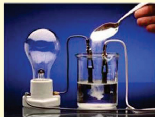
Sucrose solution, \text{C}_{12}\text{H}_{22}\text{O}_{11}(aq) non-electrolyte does not conduct electricity
