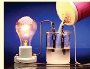
Sodium chloride solution, \text{NaCl}(aq) electrolyte conducts electricity
