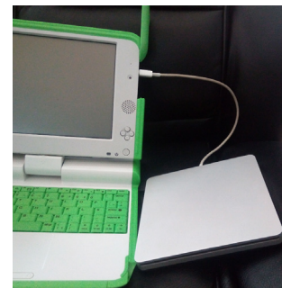
Fig. 4.7: CD reader connected to an XO laptop.
