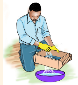
Cleaning a brick frame.
