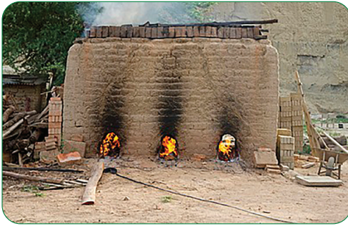
Fig. 6.5: (a) Burning bricks in a kiln
