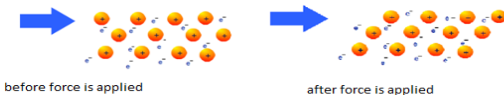
Figure 3.15 Malleability and ductility of metals
