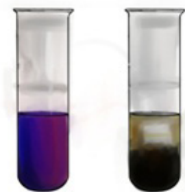
Picture 3.2: Reaction of alkenes and \text{KMnO}_4
