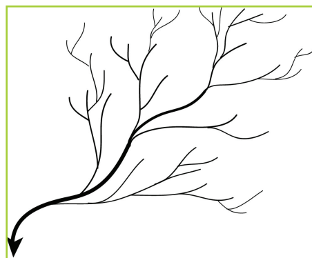
Fig 10.17 Dendritic drainage pattern.
