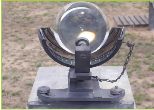
Fig 8.12 A sunshine recorder.
