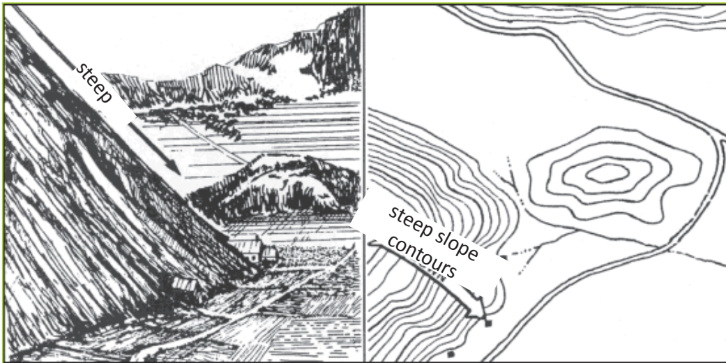
Fig 2.31 (b) Contours representing a steep slope.
