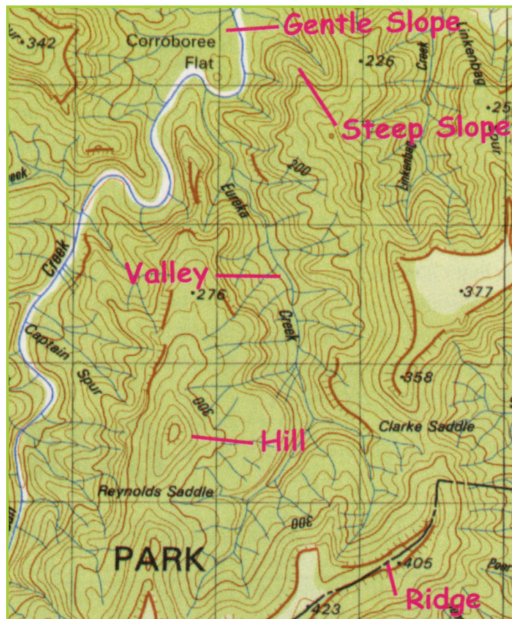
Fig 5.6 A topographic map with physical features marked by contours.
