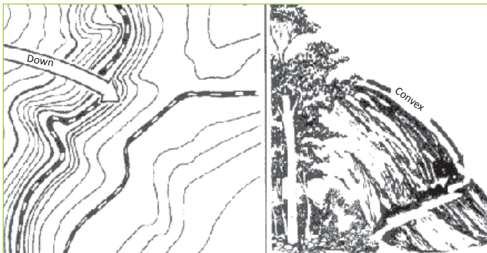
Fig 2.29 (b) Contours representing a convex slope.
