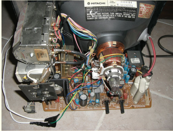
Figure 9.11: The inside of a TV set
