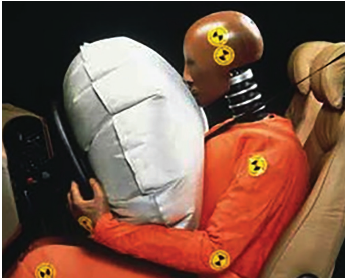
Figure 4.15: Air-bags in automobiles have saved countless lives in accidents. The air-bag increases the time interval during which the passenger is brought to rest
