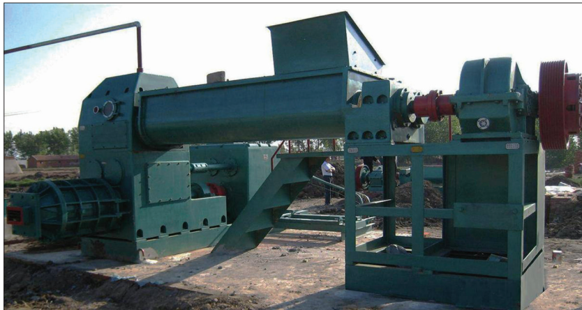
Figure 4: Machine which prepares clay in a factor.
